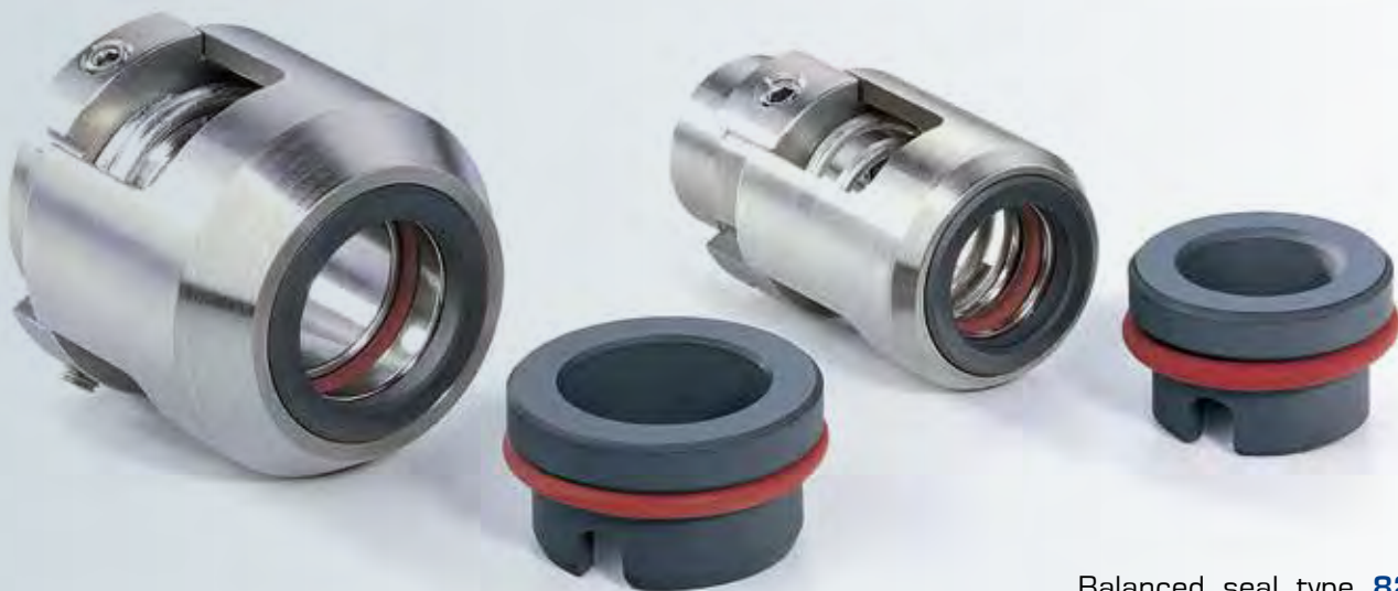
Balanced seal type 82EH for high pressure, bi-directional, all metal parts in titanium with SiC faces.
